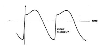
Figure 2. Distorted Forward Current in Step Recovery Diodes
