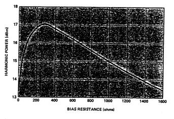
Figure 4. Effect of Bias Resistance (Second Harmonic)
