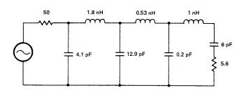
Figure 3. Optimized Lumped Element Low Pass Filter
