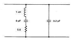
Figure 1. Diode Equivalent Circuit
