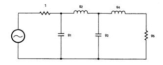
Figure 2. Low Pass Prototype for Input Filter
