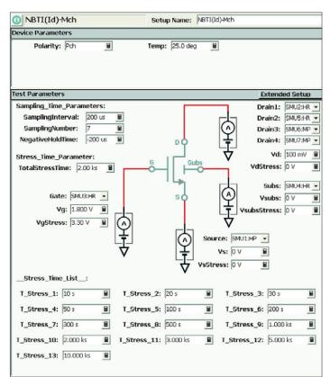
Figure 6. B1500A Multi-Channel Timing On-the-fly NBTI sample library
