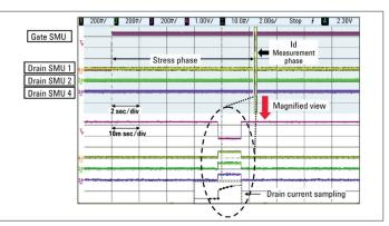
Figure 7. Waveform of the Multi-channel Timing on-the-fly NBTI test of the B1500A EasyEXPERT software
