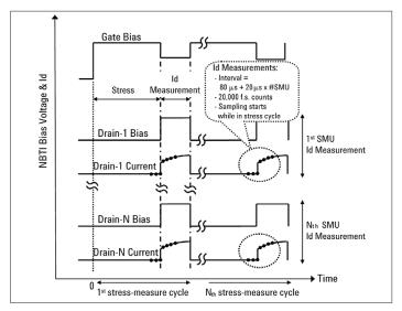
Figure 1. Multi-Channel Timing-on-the-fly NBTI test sequence and the Id measure timing
