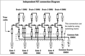
Figure 5. Device connection for multi-channel Timing-on-the-fly NBTI test
