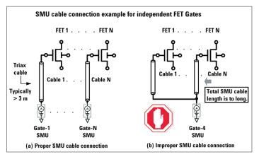
Figure 3. Tips for SMU cabling for parallel NBTI test
