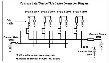
Figure 2. Device connection for multi-channel Timing-on-the-fly NBTI test
