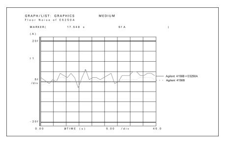
Figure 2. Noise current of the Agilent 4156A and Agilent E5250A
