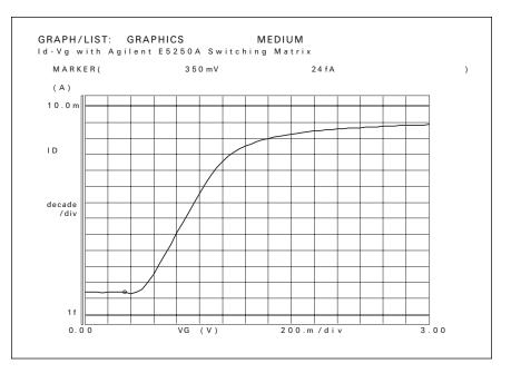
Figure 4. Id-Vg curve obtained using the Agilent 4156C with E5250A
