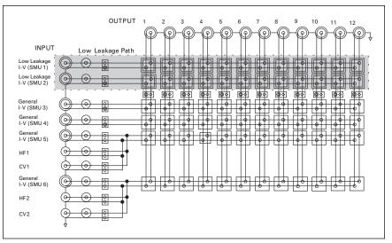
Figure 1. Block diagram of the low leakage switching matrix of the Agilent 5250A
