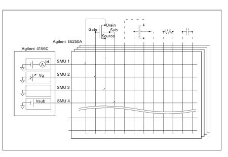
Figure 3. Measurement diagram of the Id-Vg curve of n-channel MOSFET
