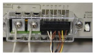
Figure 8. Power supply terminal connection
