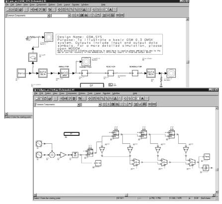
When the system-level design is complete, the synthesizable models allow you to generate HDL code efficiently.
