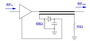
Figure 1 – Typical AGC circuit
