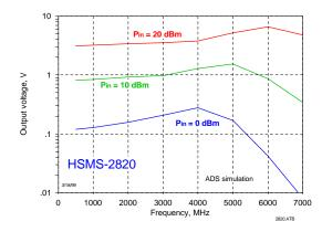
Figure 3 – simulation for HSMS-282x
