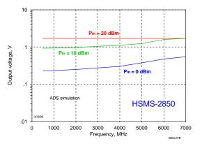
Figure 5 - simulation for HSMS-285x detector
