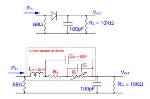
Figure 2 - Self-biased detector
