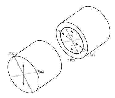
Figure 1. Model of polarization-mode coupling between birefringent fiber segments. At each equivalent fiber interface, the input wave decomposes into the polarization modes of the following segment.
