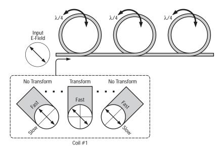
Figure 2. Fiber coil type of polarization controller. Coiling the fiber induces fast and slow linear polarization modes. The input wave decomposes into the these modes. Tilting a coil changes the decompostion, and thus the polarization transformation. The process repeats at each coil.
