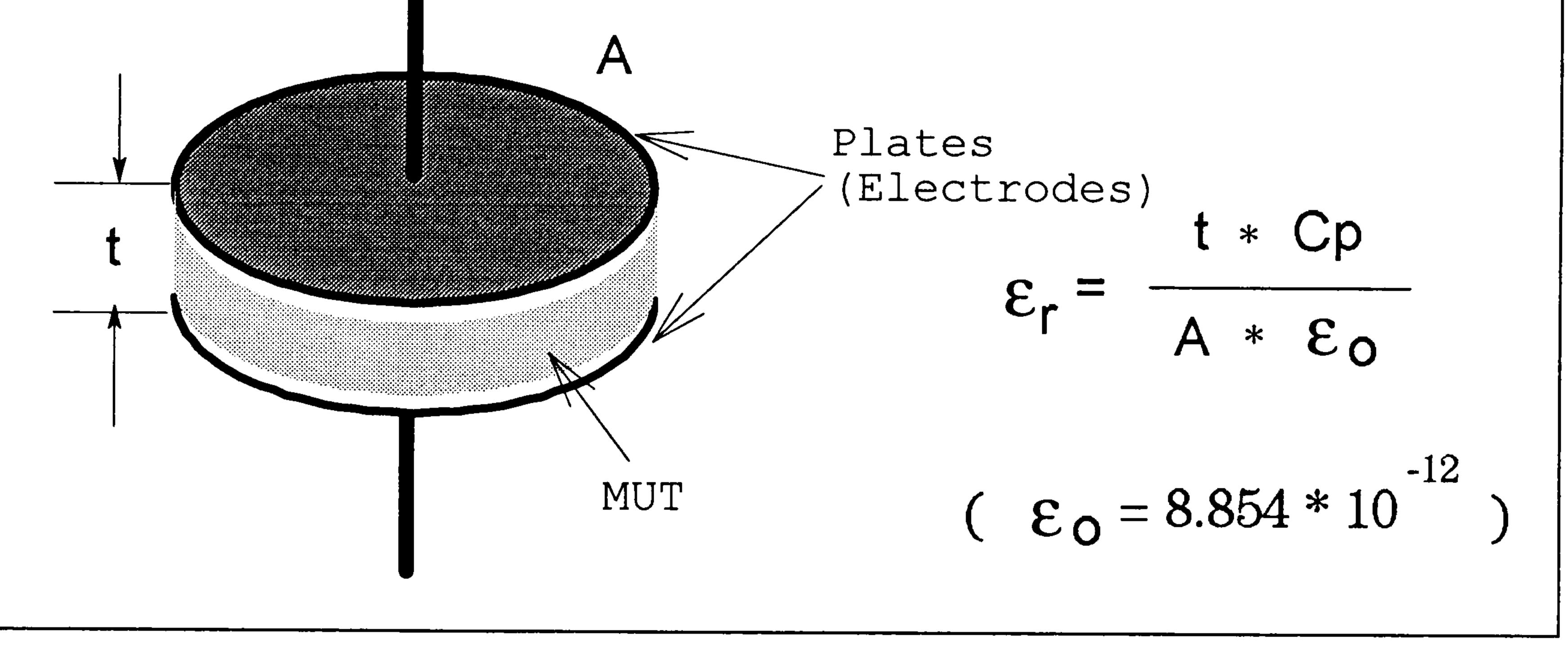
Figure 1. The Parallel Plate Method
