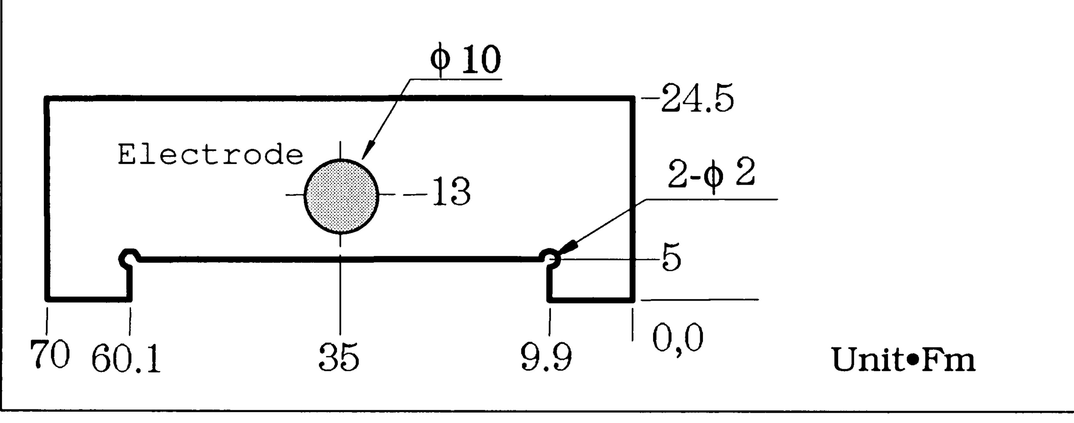
Figure 4. MUT Electrodes Shape and Position
