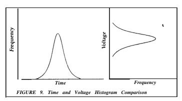
Histograms may be produced by analysis of data in either the voltage or time axis of the oscilloscope. The data for the histogram is gathered from a window defined by the user. (see figure 10). A voltage histogram will be produced from data that is gathered from a specified time interval. A time histogram will be produced from data that is gathered from a specified voltage range.
