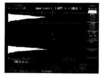
FIGURE 20. Finding the Mean One Voltage
