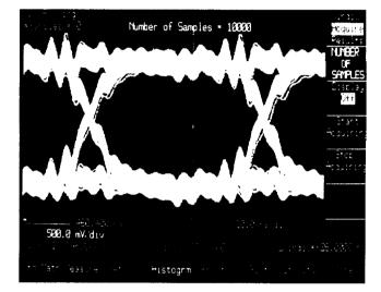
FIGURE 19. Eye Diagram and Determination of 1 and 0 Voltages
