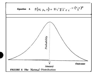
In a normal distribution, the area under the curve to the right of the positive one standard deviation (sigma) point is 15.87,7% of the total area under the curve. Therefore the area under the curve bounded by the one standard deviation points is 68.26% of the total. Similarly, the area bounded by the two and three standard deviation points is 95.44% and 99.74%, respectively.
