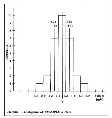
As the histogram is broken up into more and more intervals or "buckets", the histogram takes the form of a smooth continuous function. At this point conclusions may be drawn about the distribution. For instance, the distribution may be uniform, skewed, or perhaps normal as in this example. The mean and sigma are also calculated using Equations 1 and 2. Assuming a normal distribution, 68.26% of the data falls within plus or minus one sigma (0.5637 mV) of the mean (3.2770 mV).
