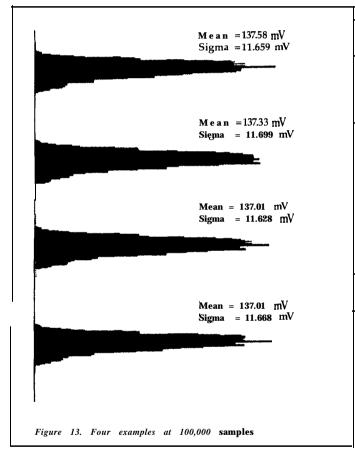
From FIGURE 13 it is apparent that the histograms have the same general shape. Also, the means and sigmas deviated very litte from one another. From trial to trial it is evident that the results are repeatable to a great extent.
