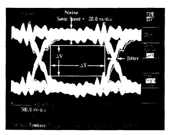
FIGURE 18. Measurements on the Eye
