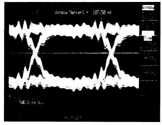
FIGURE 22. Jitter Measurement from the Eye
