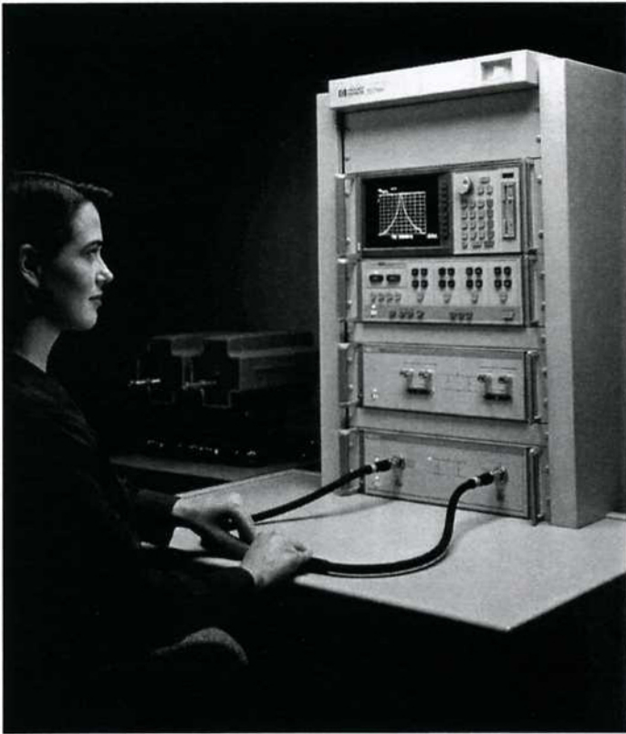
Figure 4. HP 85106D with Option 001, coaxial and waveguide capabilities all in one.
