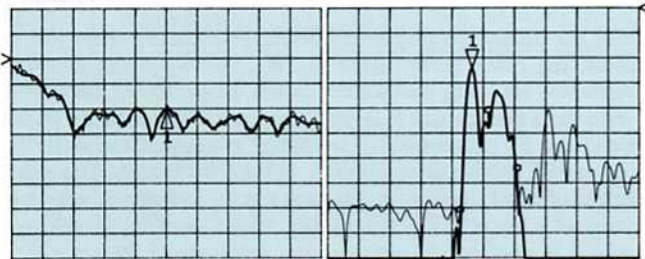
Figure 20. Calibrated RCS Frequency and Time Domain Responses of the Brass Cylinder Turned 45° Using the 1-Port RCS Calibration Procedure.
