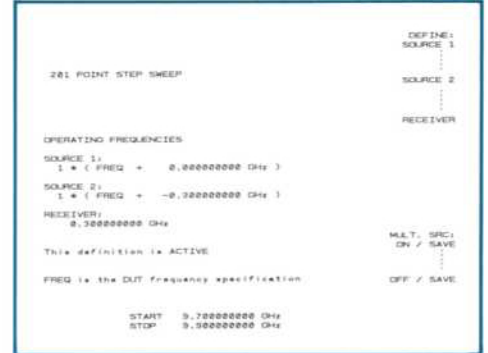
Figure 9. Multiple Source Mode Frequency Definitions for Measurement of Dual-Channel Receiver.
