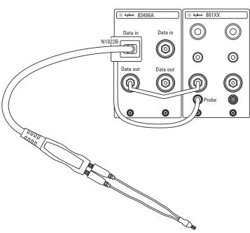
Figure 4: Connector scheme using the 83496A/B and N1022B
