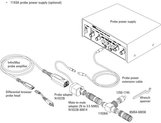
Adapting and splitting signals for probing and clock extraction with the 83496A/B option 101
