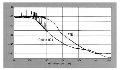
Typical SSB phase noise and spurs at 1 GHz in digitized FM
