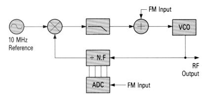
Figure 1. Simplified Agilent 8644A/65A block diagram
