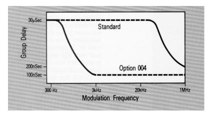
Figure 2. Group delay for digitized FM synthesis
