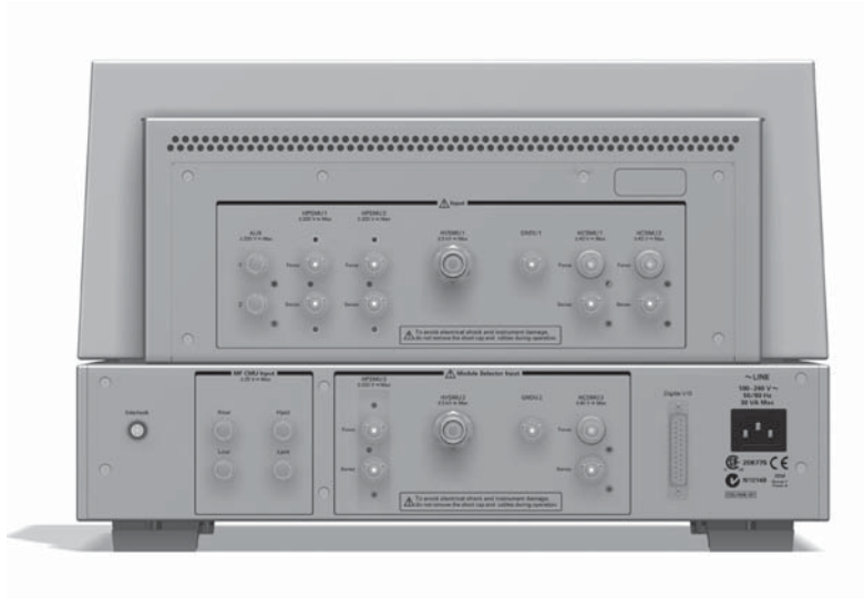
Figure 3.50. The N1259A high power test fixture mounts on top of the N1259A-300 module selector unit for packaged device testing.
