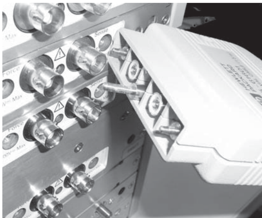
Figure 2.18. The Kelvin triaxial cable mates with Agilent SMUs and many analytical wafer prober connector plates.
