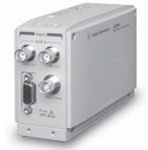
Figure 4.18. The inputs to the ASU, showing the two coaxial inputs (top), the triaxial input (from the force line of the HRSMU, lower right) and the control cable input (also coming from the HRSMU, lower left).
