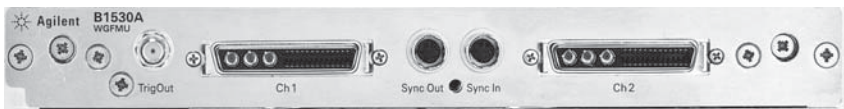
Figure 5.24. The B1500A’s WGFMU module can output 10 V peak-to-peak and has a minimum pulse width of 100 ns.
