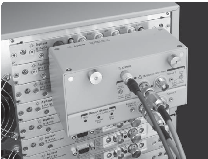
Figure 4.20. A picture of the SCUU mounted on the rear of the B1500A to illustrate how the MFCMU and SMU outputs are converted into two sets of triaxial outputs (force and sense).
