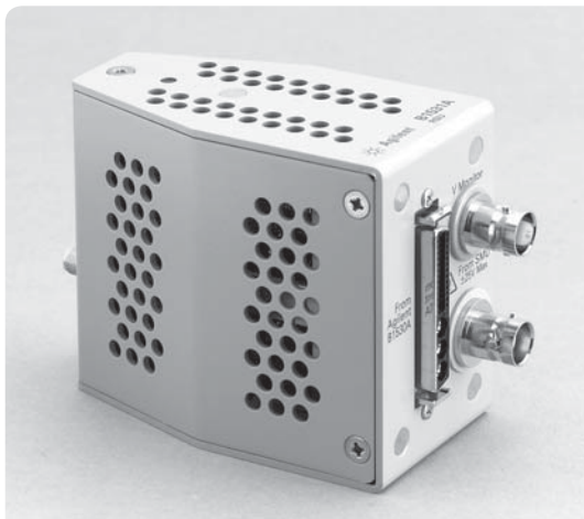
Figure 5.28. A photograph of the RSU module showing its voltage monitor (coaxial) output, SMU (triaxial) input and connector input for the cable that goes to the WGFMU module.
