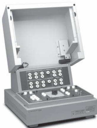
Figure 3.48. The Agilent N1259A High-Power Test Fixture provides a safe and supported solution for testing power devices at up to 20 A and 3000 V.
