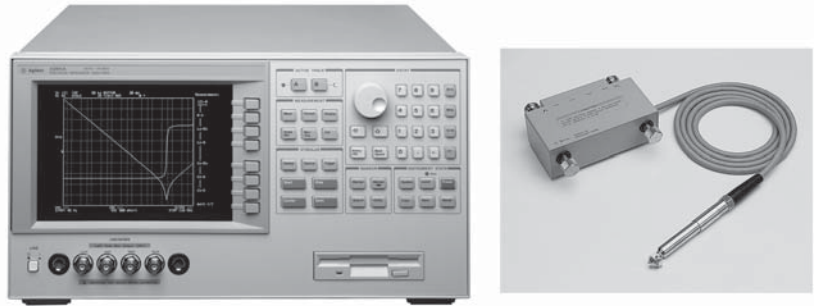
Figure 8.36. The 4294A precision impedance analyzer and the 42941A impedance probe are both required to perform the advanced IV method of CV measurement.
