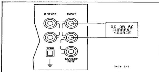
Figure 3-2. Typical Input Measurement Connection
