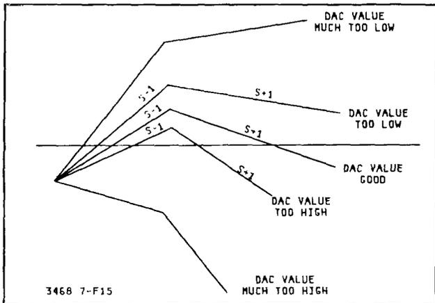
Figure 7-F-15. Determining the DAC Setting
