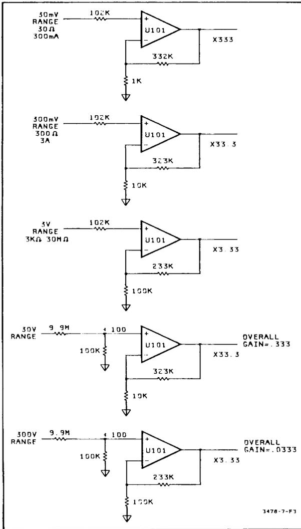
Figure 7-F-3. Simplified Schematic Of The DC/Ohms Input Amplifier
