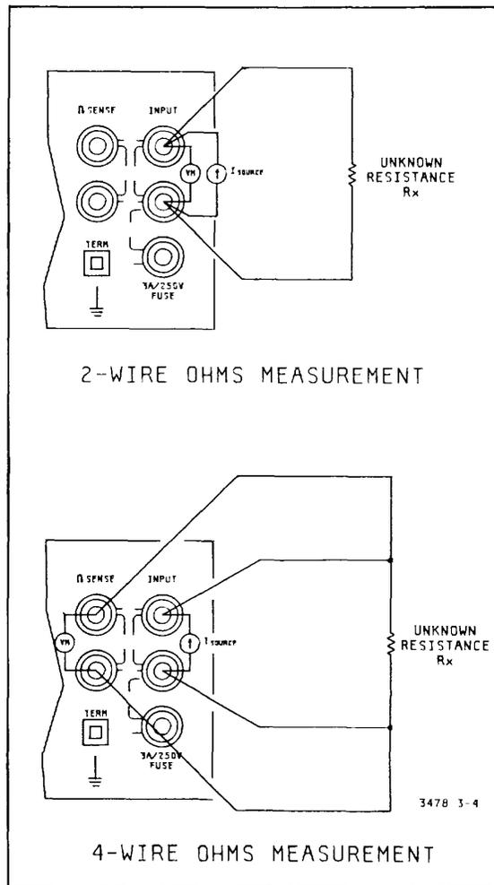
Figure 3-4. Ohms Connections
