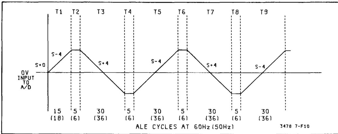
Figure 7-F-10. Runup Slopes for Zero Inputs (41/2 Digit Model)
