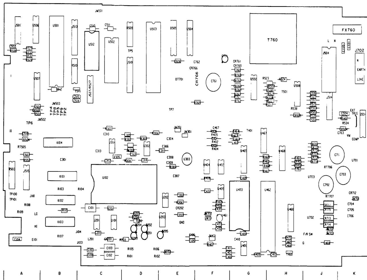
Component Locator for Input Circuitry and Ohms Current Source
