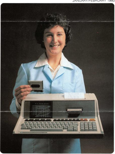
The HP-85 computer weighs a mere 20 pounds (9 kilograms). It's a very BASIC computer designed for individual use, with interactive graphics, expandable memory, optional peripherals, and interfacing potential disproportionate to its modest price.
