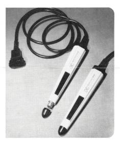
This new HEDS-3000 Digital Bart Code Wand is designed to scan black-and-white bar code and output TTL and CMOS-compatible signals. The heart of the wand is an advanced, high-resolution, high-speed, emitter/detector sensor in a sealed module near the removable tip.
