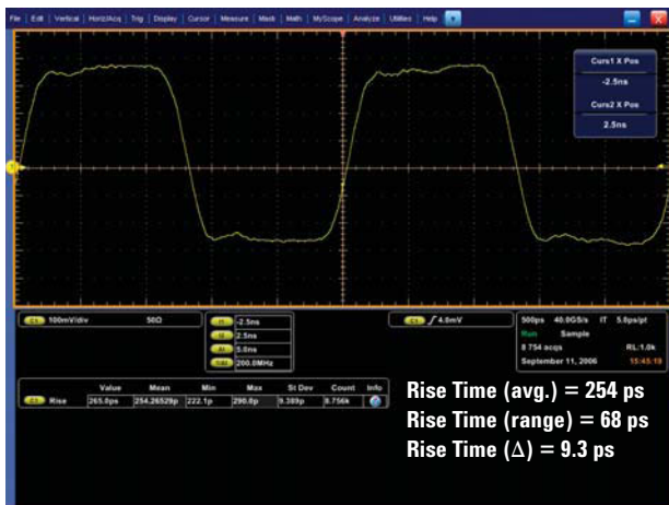
Figure 5b. 400-MHz clock captured on a competitor's 2.5-GHz oscilloscope sampling at 40 GSa/s.
