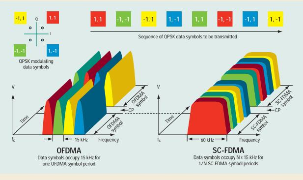
Figure 2. Comparison of how OFDMA and SC-FDMA transmit a sequence of QPSK data symbols
