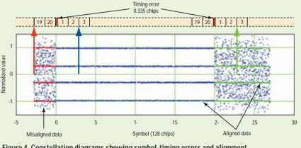
Figure 4. Constellation diagrams showing symbol-timing errors and alignment
