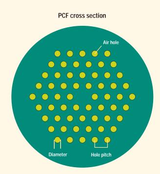
Figure 3. Conventional hexagonal photonic crystal fiber (PCF), shown in cross section, can be applied to the design of terahertz dielectric waveguide.<sup>2</sup>
