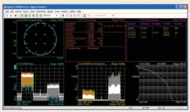
Figure 5. Analysis of a 16QAM SC-FDMA signal
