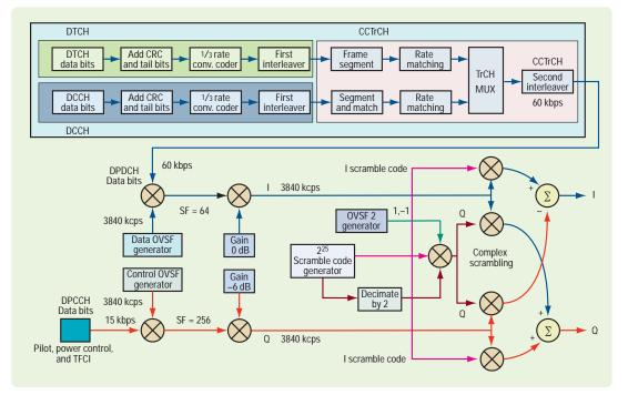
Figure 1. Uplink data-channel air interface
