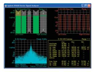
Figure 2. In this analysis of a demodulated RFID signal, bursts are identified with down arrows representing interrogator bursts and up arrows indicating tag return transmissions. Note that tag amplitude levels are well below those of the reader.
