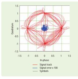
Figure 8. Typical W-CDMA modulation waveform results for 30 traces (red). The error between different results sets is < 0.25 percent (blue).
