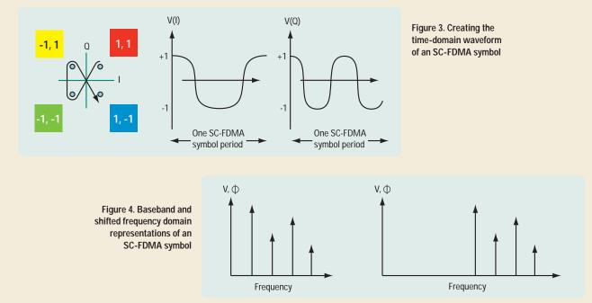
\*Although 3GPP did consider a distributed form of subcarrier allocation for the uplink that would have alleviated susceptibility to narrowband fading, it instead opted for the adjacent allocation described here combined with the possibility of frequency hopping at the slot (0.5 ms) level.
