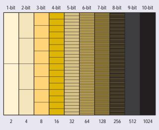
Figure 2. Resolution quoted as bits indicates the number of discrete measurement levels used.
