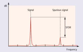
Figure 6. Spurious-free dynamic range affects the usable dynamic range in a measurement.
