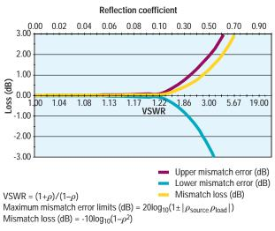
where  $\rho$  = reflection coeficient and  $\rho_{\rm source}$  =  $\rho_{\rm load}$
