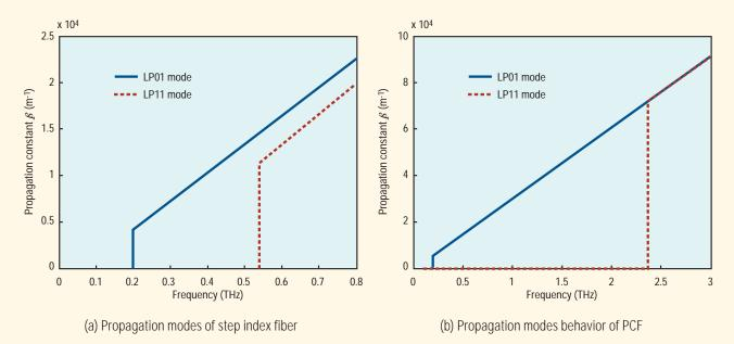
Figure 4. These diagrams enable a comparison of mode behaviors: (a) Propagation modes of step index fiber,  $n_{care} = 1.45$ ,  $n_{clad} = 1$ , r = 0.21 mm; (b) Propagation modes of PCF,  $n_{core} = 1.45$ , air hole diameter d = 0.350 mm, air hole pitch  $\Lambda = 0.725$  mm.
