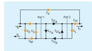
Figure 2. The systematic errors shown in Figure 1 are described here by the 12-term error model flow graph. There is one flow graph for the forward direction (six terms shown here) and another for the reverse direction (six more terms).
