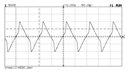
12. If the waveform is symmetrical the limiting action is working and no further verification is required.
