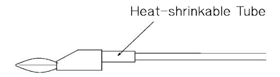
Figure 1. Improved Cable Assembly
