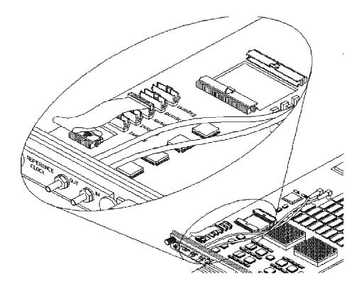
If only three connectors are present (J5-J7) as shown in the following figure, then the board is not to be replaced.
