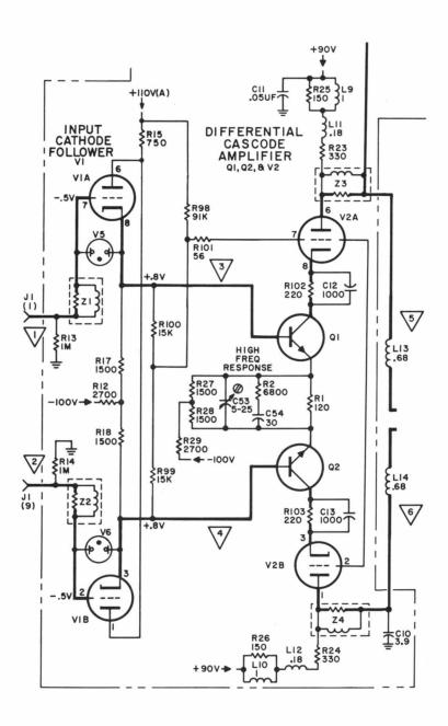
Figure 1. HP Model 175A Oscilloscope, Schematic of Modified Circuit
