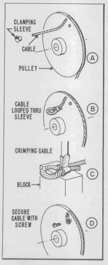
New type cables are constructed of plastic coated copper woven wire with a stainless steel core, and cannot be satisfactorily soldered.
