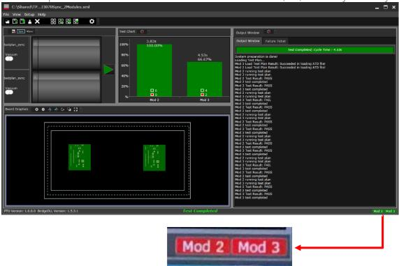
A parallel test feature license is required in each of the VM for ICPT to establish control to its BT Basic windows. However, this feature license is only support at i3070 software version 10.0p and above. Without this license, ICPT will not be able to detect the modules.
