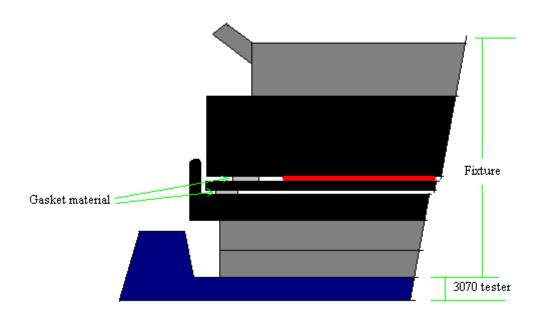
In addition to this potential fingertip pinch hazard, other finger pinch hazards may also exist on these or other fixtures in use on Agilent 3070 systems. For more information regarding other potential hazards, reference the following documents located on the Agilent Technologies website:
