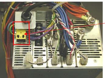
Figure 1. Cable harness side of the MPU.
