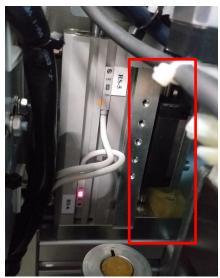
Figure 1: Runner Block and Rubber support hard-stop.
