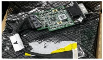
Figure 3a: Adapter-Card RS232A Srl SPS-Power (Keysight P/N: 0960-3630)
