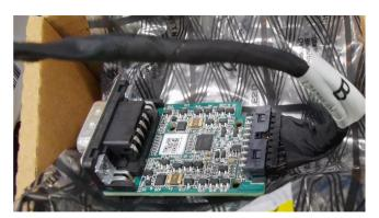
Figure 3b: Adapter-Card RS232B Srl SPS-Power (Keysight P/N: 0960-3629)
