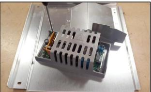
Connect Power Supply Cable (5041-5251) to the Power Supply and the PCB Main Board Assembly.
