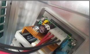
Re-attach the line power connectors, being careful to get the orientation of the connectors correct.
