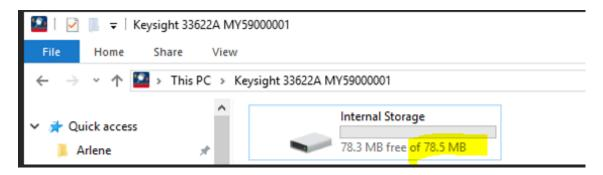
If the internal storage size of your 33611A waveform generator is 78.5MB instead of 970MB, please return the instrument to the nearest service center for repair.
