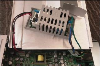
Disconnect the power input and output connectors and remove the four screws holding the power supply to the swing out panel.
