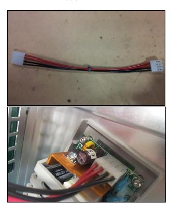
Re-attach the line power connectors, being careful to get the orientation of the connectors correct.
