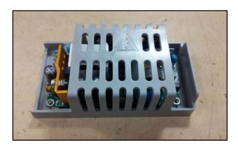
Assemble the Power Supply Shield with the Power Supply in it to the Power Supply Deck as shown. Make sure the orientation of the powers supply is correct. Secure the four screws (0515-0430) to the Power Supply Deck by using T10 Torx as shown below.
