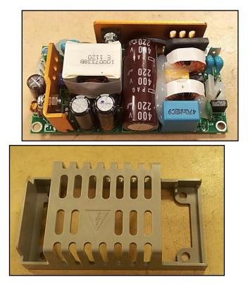
Assemble the new Power Supply into the Power Supply Shield by sliding the power supply into the shield. Note the orientation of the power supply needs to be correct, where the highlighted capacitor needs to be clearly visible.
