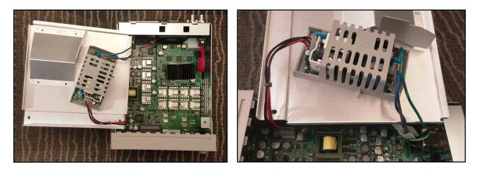
Disconnect the power input and output connectors and remove the four screws holding the power supply to the swing out panel.
