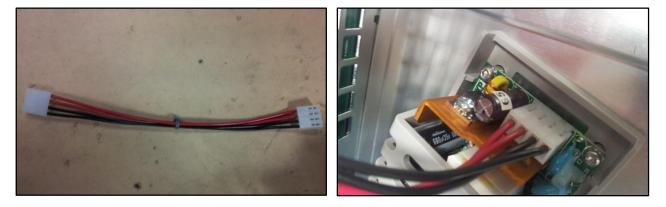
Re-attach the line power connectors, being careful to get the orientation of the connectors correct.
