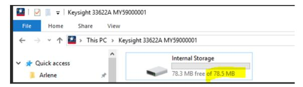
If the internal storage size of your 33621A waveform generator is 78.5MB instead of 970MB, please return the instrument to the nearest service center for repair.
