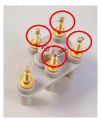
Contact the nearest Service Center for repair if similar failure persists after adding solder to the shorting block.
