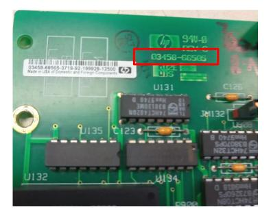
If the firmware revision is not 9,2 or the instrument has a 03458-66505/03458-66515 A5 Outguard Logic PCA, you will need to order a new A5 Outguard Logic PCA (03458-66675) and cable (03458-61611) in addition to the A3 A/D Converter PCA to complete the repair. The 03458-66675 PCA updates the instrument firmware to 9,2.
