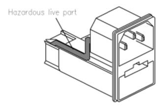
Figure 1. AC Line Connector
