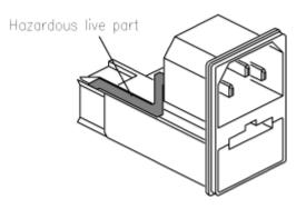
**Figure 1. AC Inlet Connector**
