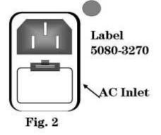
Figure 2. Repair Completed Label
