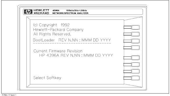
Figure 1. Bootloader Screen
