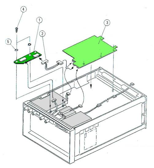
Figure 1 Filter board replacement
