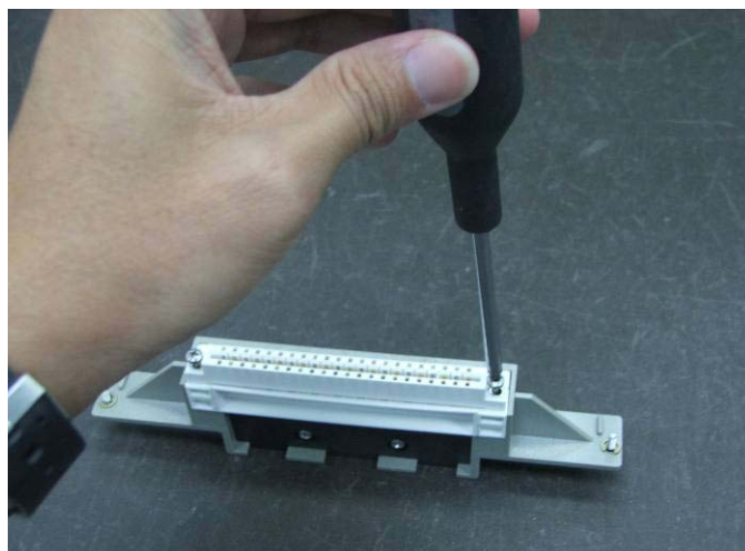
Figure 5: Good Connector attached to terminal block
