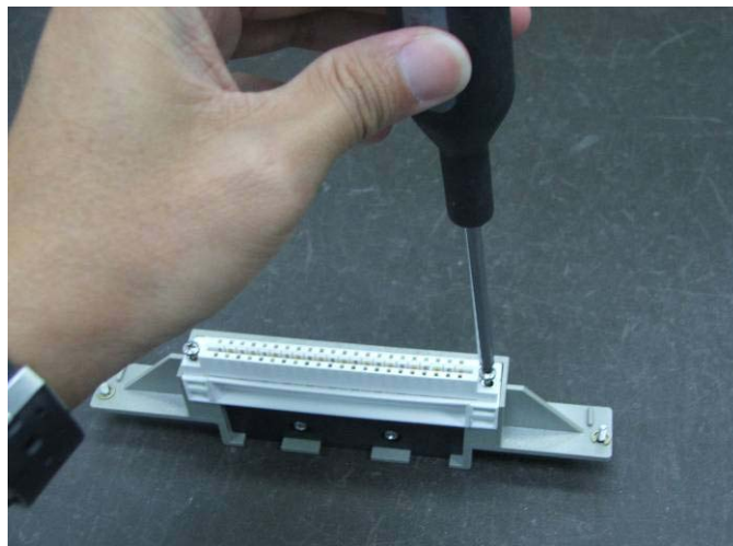
Figure 5: Good Connector attached to terminal block
