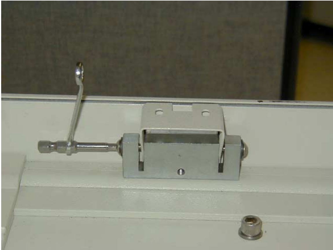
Figure 6. Installing the Tamper Proof Screws.
