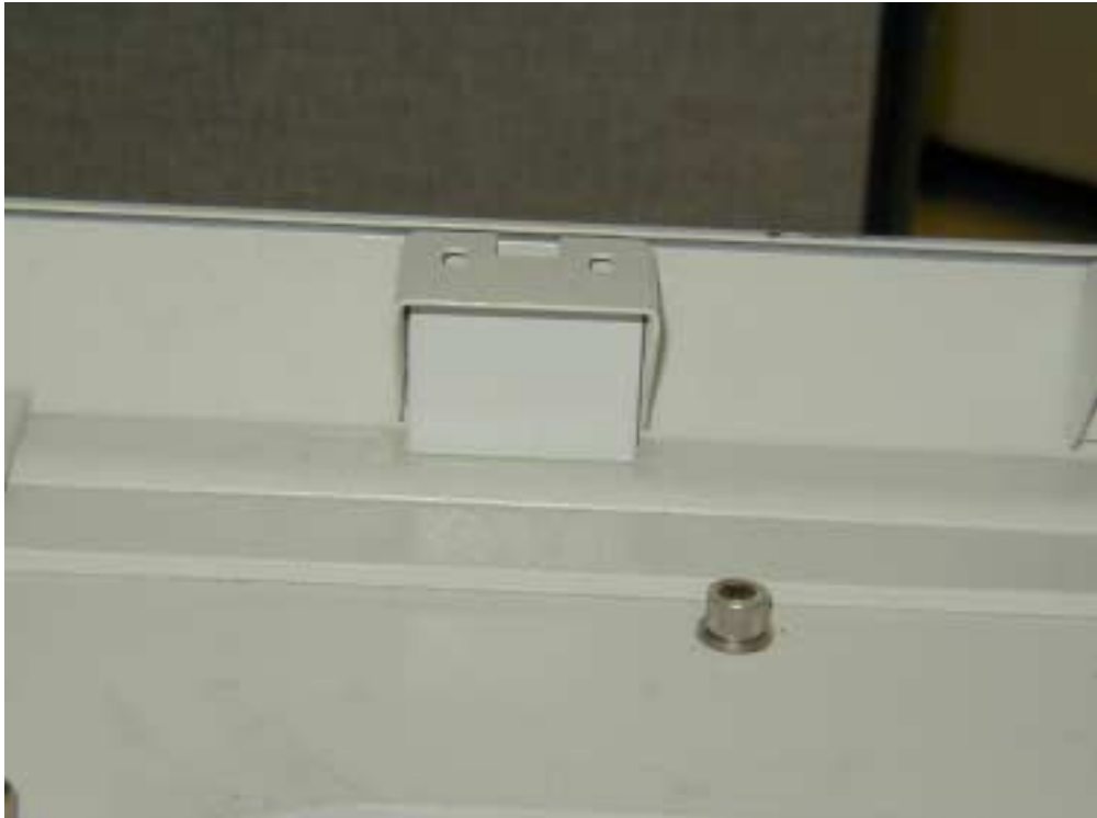
Figure 3. 5DX with new Lead Shield installed
