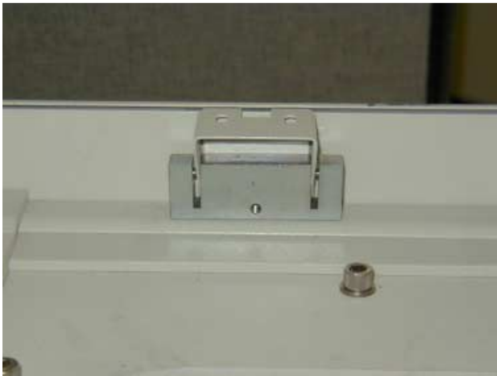
Figure 5. 5DX with new Lead Shield and Clamp Installed.
