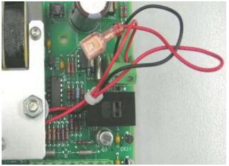
Figure 14 (New Control board with voltage regulator)
