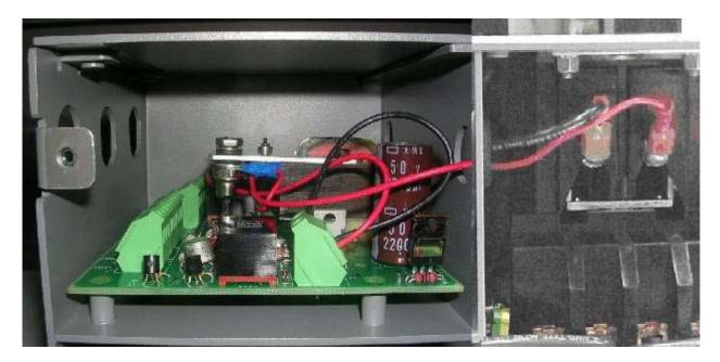
Figure 15 (new Control Board with voltage regulator)
