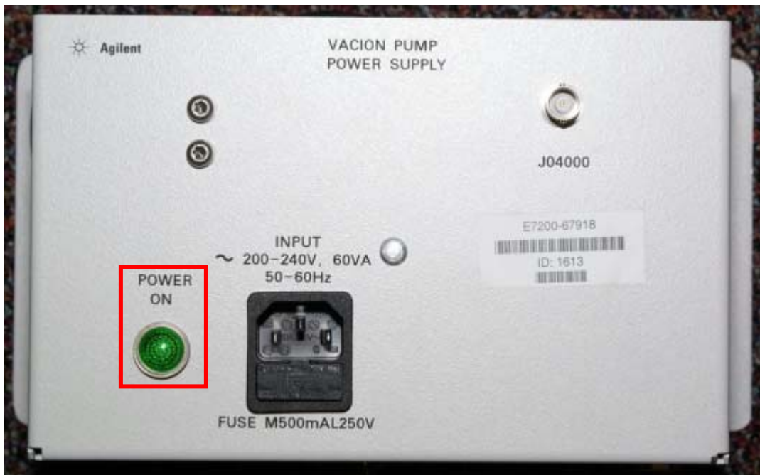
Figure 1: Green Lamp Indicator on Vac Ion Power Supply
