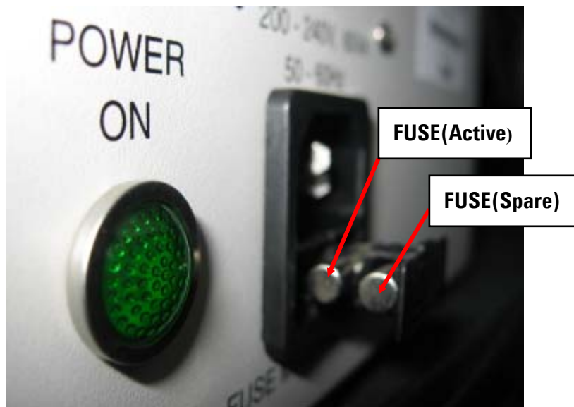
Figure 2: Fuse Compartment on the Vac Ion Power Supply
