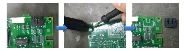
2. Remove the wires from the housing that mated with the connector at J206.
