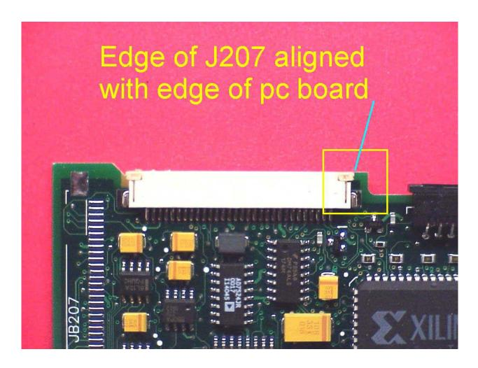
**CORRECT J207 PLACEMENT** – alignment to within < 0.3mm Picture shows connector aligned to edge of SMT board to within <0.1mm
