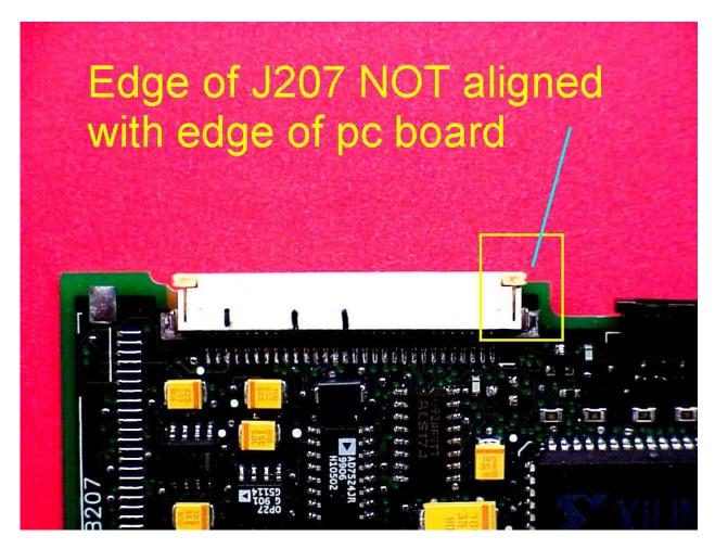
**INCORRECT J207 PLACEMENT** – misaligned by > 0.3mm Picture shows connector extending past edge of SMT board by >1.2mm
