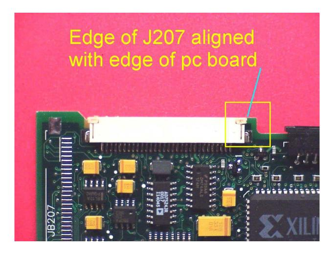
**CORRECT J207 PLACEMENT** – alignment to within < 0.3mm Picture shows connector aligned to edge of SMT board to within <0.1mm
