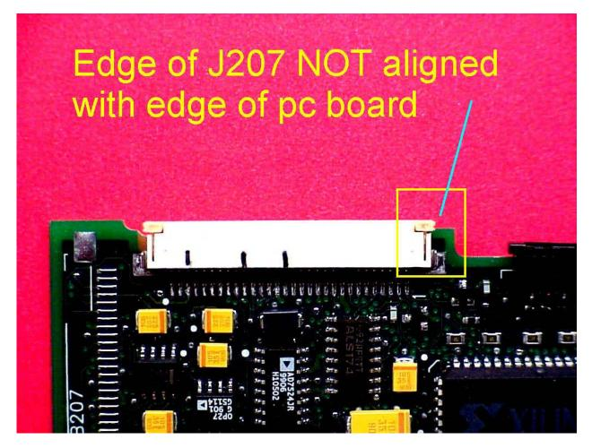
**INCORRECT J207 PLACEMENT** – misaligned by > 0.3mm Picture shows connector extending past edge of SMT board by >1.2mm
